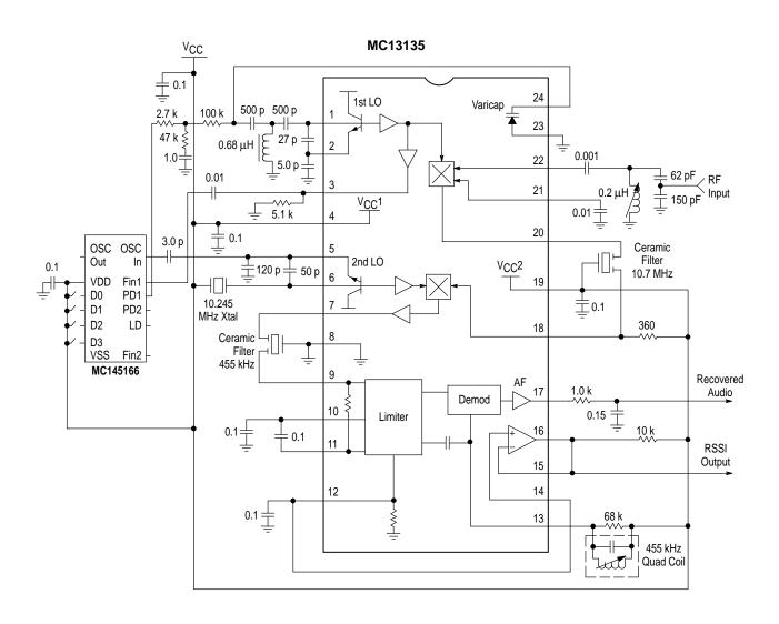
Figure 16. 144 MHz Single Channel Application Circuit
