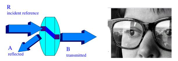
Scatter Parameters, also called S-parameters, belong to the group to twoport parameters used in twoport theory. Like the Y or Z parameter, they describe the performance of a twoport completely. Different to Y and Z, however, they relate to the traveling waves that are scattered or reflected when a network is inserted into a transmission line of a certain characteristic impedance ZL. Therefore, S-parameters can be compared to reflection and throughpass of a pair of spectacles.
