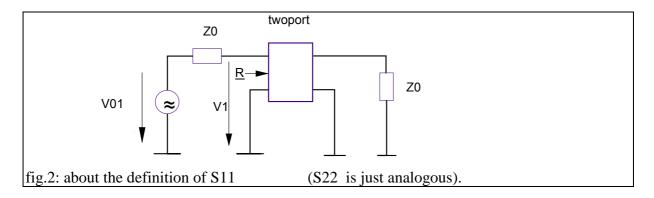
Under the assumption that  $\underline{R}$  is the complex input resistance at port 1 and Z0 is the system impedance, we get using eq.(2) and the resistive divider formula:
