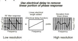
Fig.5: Applying electrical delay
