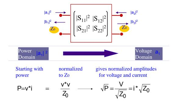
In other words, we can convert the power towards the twoport into a normalized voltage amplitude of
