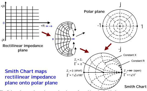
Fig. 3: how the complex resistance plane is transformed into the Smith chart
