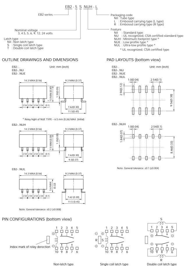
S : Coil polarity of set (operate)
